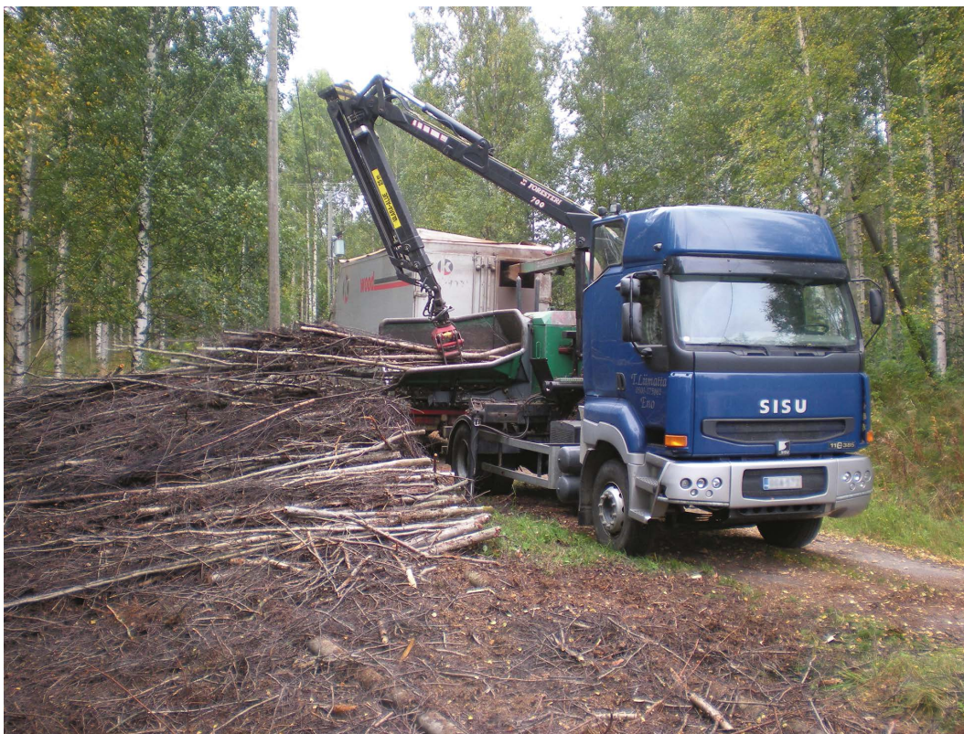
Figure 13. Chipping at the roadside. Photo: Antti Asikainen.
